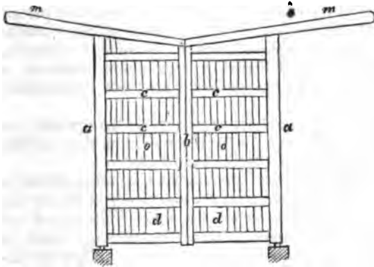
Fig. 173— Represents the elevation of a lock-gate closed.
